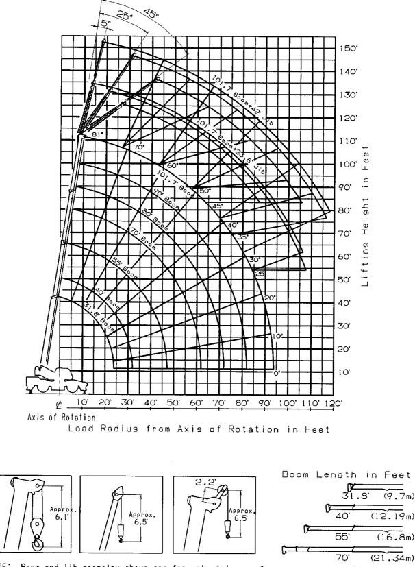
NOTE: Boom and jib geometry shown are for unloaded condition and machine standing level on firm supporting surface. Boom deflection and subsequent radius and boom angle change must be accounted for when applying load to hook.
