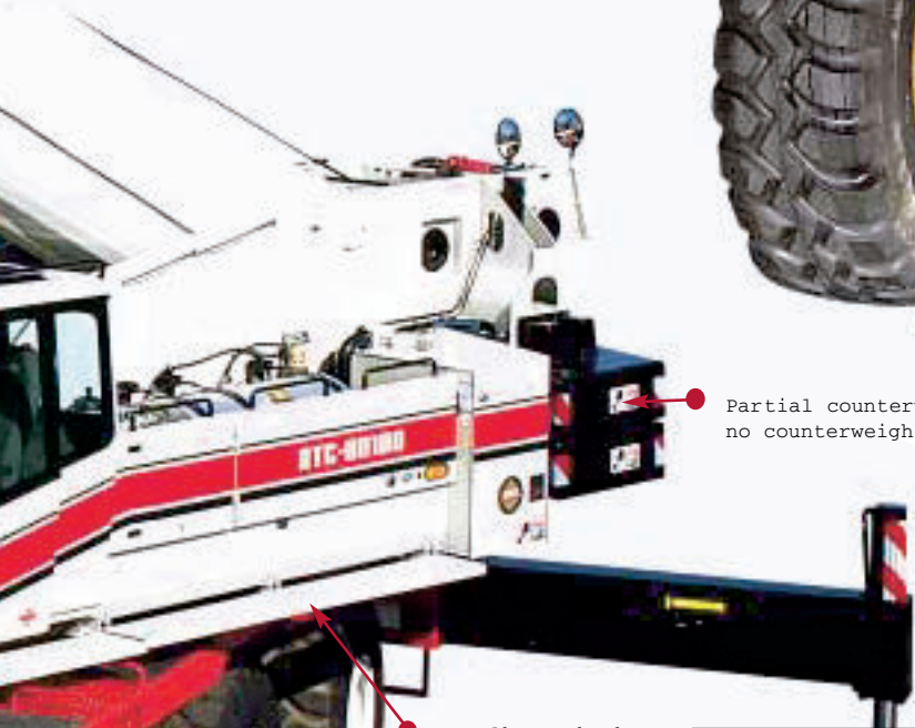
Catwalks on both sides of upper
