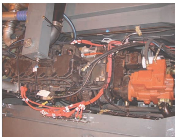
Cummins QSB 6.7L diesel engine provides plenty of power at the jobsite and meets current emission standards.
