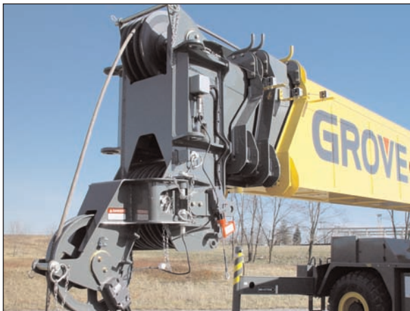
The RT530E-2 incorporates a rectangular boom shape made from 100k.s.i. steel which eliminates weight and maximizes structural capacities.
