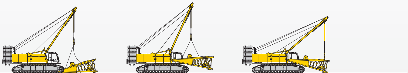
Unloading and assembly of boom foot
