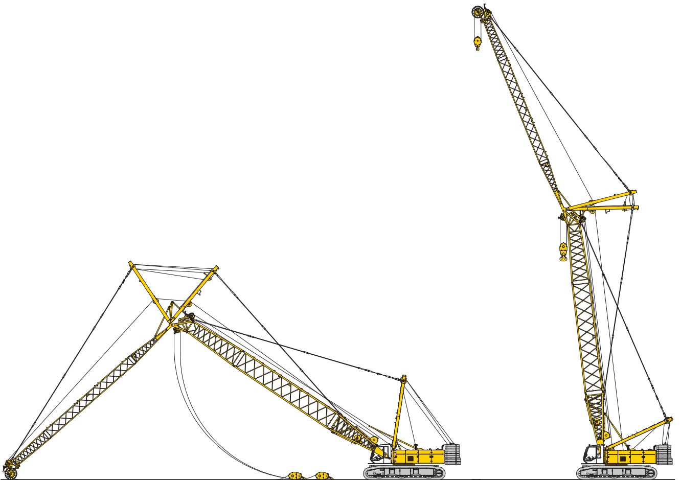
Erecting of main boom and luffing jib
