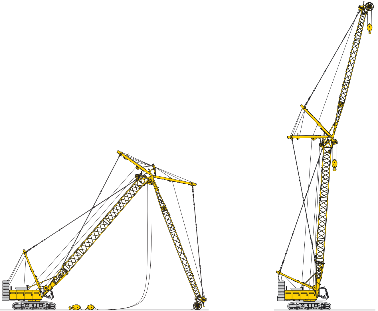
Erecting of main boom and luffing jib
