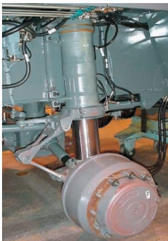
MEGATRAK™ Independent suspension and all-wheel steer system allows wheels to remain on the ground at all times so stresses and weight are not continually transferred between axles.
