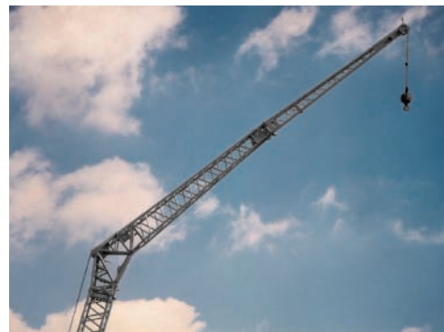
LUFFING BI-FOLD SWINGAWAY Hydraulically offset lattice bi-fold swingaway lets the operator set the offset from 0°-40° while under load from the superstructure cab
